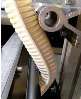
and bending tests show how flexible the e-skin® soft cables, even under loads that would break other cables
