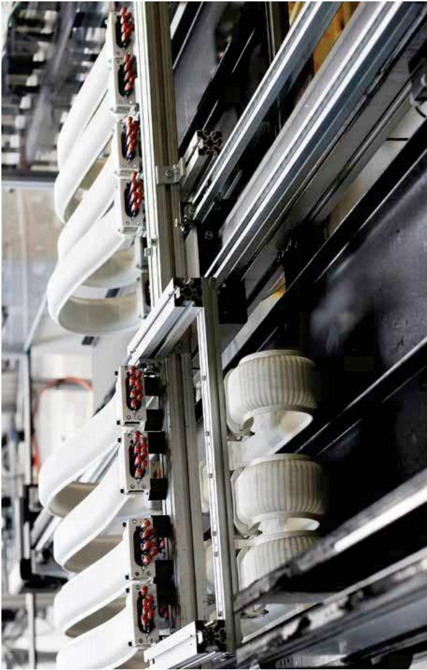
Service life test in the 3,800m² igus® laboratory in Cologne (Germany)
