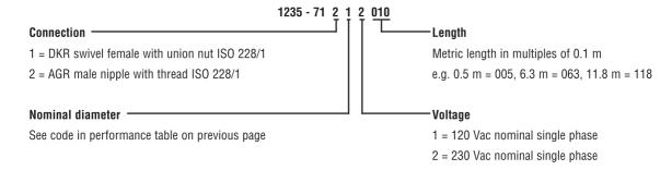
Example: 1 m heated hose, 4 mm nominal diameter, 230 V supply voltage, AGR connection
