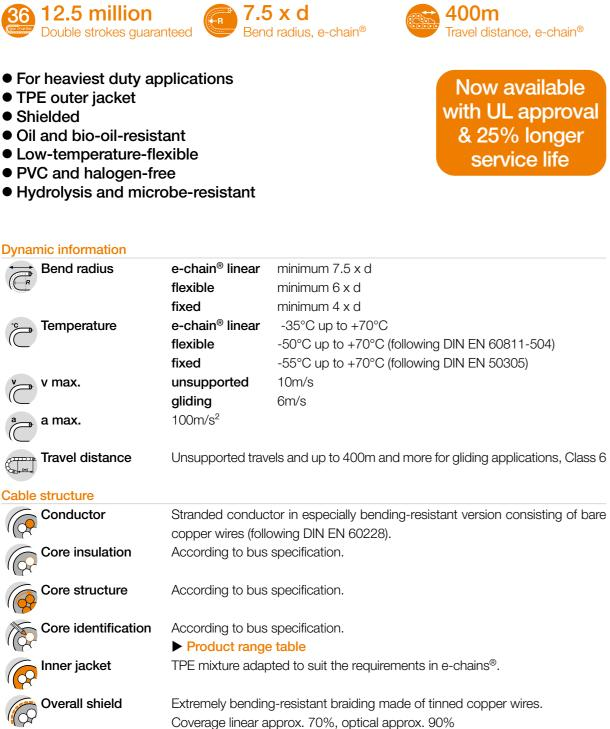
Extremely bending-resistant braiding made of tinned copper wires. Coverage linear approx. 70%, optical approx. 90% Outer jacket Low-adhesion, extremely abrasion-resistant and highly flexible TPE mixture, adapted to suit the requirements in e-chains®. Colour: Red lilac (similar to RAL 4001) Variants <a>Product range table</a>
