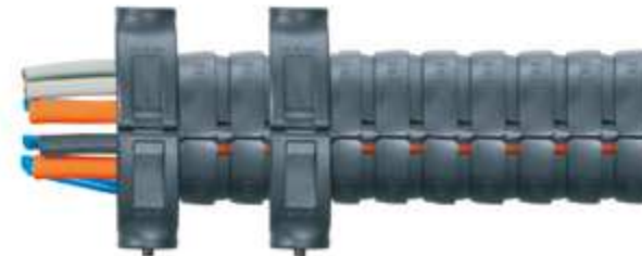
Mounting bracket without strain relief (recommended on axes 1 - 3 to provide length compensation for cables and hoses)
