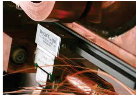
Due to the welding spatter and dust, the use of the extremely dirt-resistant drylin® T linear guide finds the balance between high service life and low costs.
