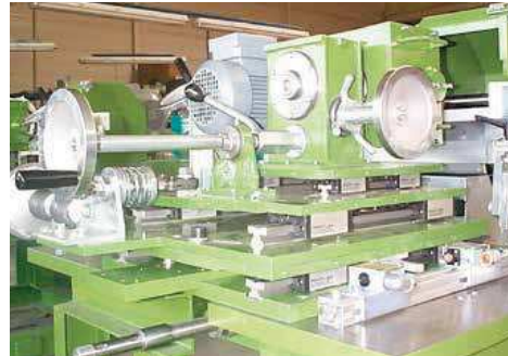
The adjustment of the pressing roller and the compensation of the imbalance of the grinding tools are implemented with drylin® T in place of recirculating ball bearing guides.
