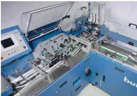
The drylin® T linear guides are used in these enveloping machines to guide an envelope suction opener that is mounted on one side.
