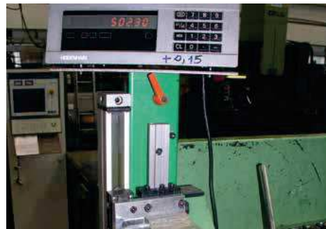
Time saving: Reduced tool changing time due to this measuring system. The gauge is guided on a drylin® T rail. This solution works also without problems in dusty environments.
